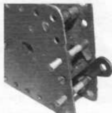
1\frac{1}{2} " axles as locating dowels.
