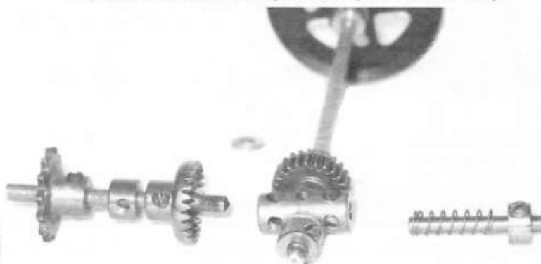
Picture 109 – Reduced MO Motor output shaft from inside boiler. From left to right. On a 2" Axle Rod is \frac{3}{4} " Sprocket Wheel, Collar, \frac{3}{4} " Contrate Wheel. Then on a 5\frac{1}{2} " Axle Rod, a Collar, Washer, Coupling, 2 x Washers and \frac{3}{4} " Pinion. The 2" Pulley is from inside the firebox. Then on a 1" Axle Rod, a Compression Spring and Collar to hold everything in place.
