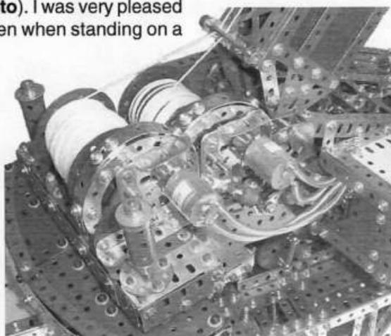
The crane hoist drums and drive
