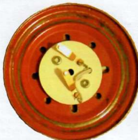
Bruce Geange's version of the Ball Thrust Bearing commutator (please refer to page 8)
