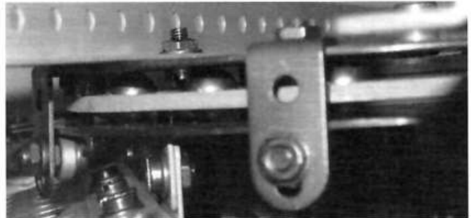
The turntable showing inner ball rollers and outer hook rollers.
