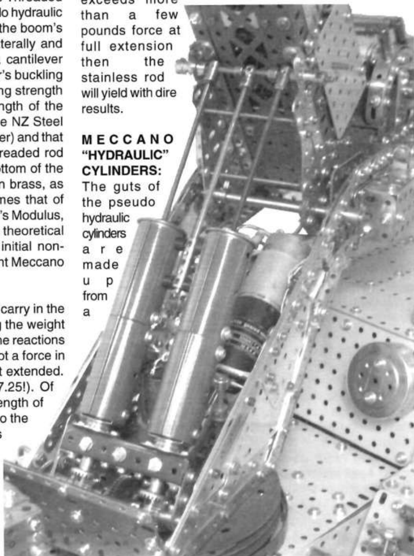
Figure 1: Overall View of Luffing Cylinders, boom at 70-degrees. Brass Thrust Bearings visible below blue cylinders.
