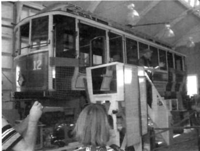
On the left is Lou Nichols' photo of the Tramcar No 12 - up on a steel supporting frame waiting for the wheels and driving motors to be fitted.
