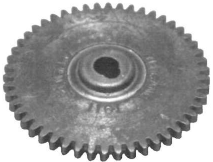
Fig.1 - c1911 50 tooth gear with tunnel keyway
