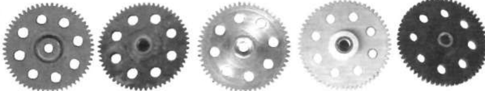
Fig.2 - Range of 57t gears from c1924 on left to modern plastic versions to right.
