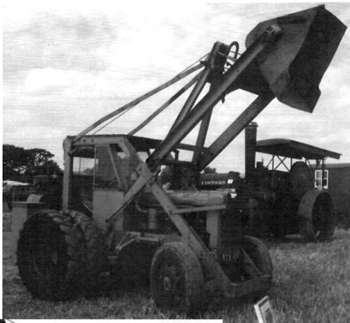
Figure 5 shows the Chaseside loader with the bucket elevated.
